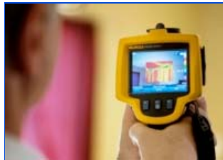
A thermal imager shows an infrared image and the varied temperature of an exterior wall as Jon Traudt, certified by the EPA to inspect homes for energy efficiency, inspects an Omaha home.
